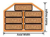
Dimensional Measurement of CTC is done on straight specimen of approximately 400mm length with open ends under a pressure of 1 N/mm2.
